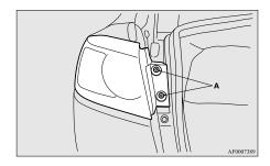
2. Remove the lamp unit in the rear direction.
