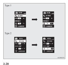
3. Press and hold the multi-information meter switch for about 2 seconds or more to switch in sequence from  ${}^{\circ}C \rightarrow {}^{\circ}F \rightarrow {}^{\circ}C$ .
