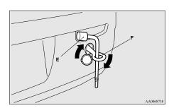
4. Always attach the tow rope to the towing hook. Otherwise, the instructions are the same as for "When being towed by another vehicle".
