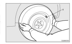
7. Finger-tighten the wheel nuts.
