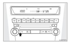
Push the CD button (2) if a disc is already in the CD player. The audio system will enter CD mode and start playback. The track number and the playing-time will appear on the display. The tracks in the disc will be played consecutively and continuously
