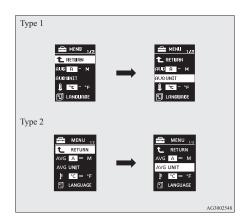
Press and hold the multi-information meter switch for about 2 seconds or more to display "AVG UNIT" (fuel consumption display unit setting).
