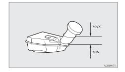
The fluid level is monitored by a float. When the brake fluid level falls below the "MIN" mark, the brake fluid warning lamp lights up.
