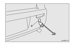
3. Use the wheel nut wrench (E) to firmly attach the towing hook (F).
