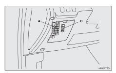
A- Main fuse block B- Sub fuse block 1. Open the fuse lid and pull to remove it.
