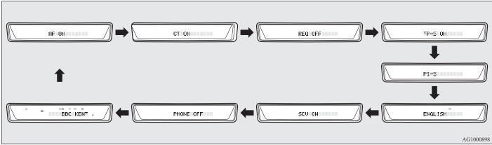
3. Press the TUNE switch (B) repeatedly to select the CT (Clock Time) mode.
