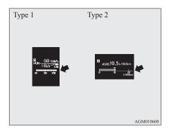
When the momentary fuel consumption surpasses the average fuel consumption, the momentary fuel consumption is displayed with a green bar graph. (Type 2)
