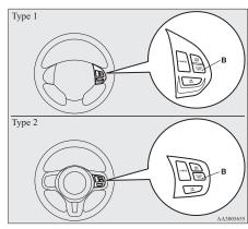
To slow down your speed in small amounts, press the "COAST SET" switch for less than about 1 second and release it.
