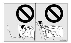
Use rearward facing child restraints in the rear seat or turn off the front passenger's airbag ON-OFF switch (if so equipped). (Refer to "To turn an airbag off" on page 2-24.)
