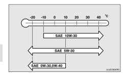
Select engine oil of the proper SAE viscosity number according to the atmospheric temperature
