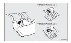
2. Release the clutch pedal. The "ASSG" display/indicator will turn on and the engine will stop automatically.
