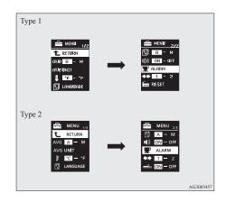
Press and hold the multi-information meter switch for about 2 seconds or more to switch in sequence from 1 (turn-signal sound 1) → 2 (turn-signal sound 2) → 1 (turn-signal sound 1).
