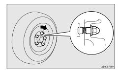
Steel spare wheel Tighten the wheel nuts until the tapered parts of the wheel nuts make light contact with the seats of the wheel holes and the wheel is not loose.
