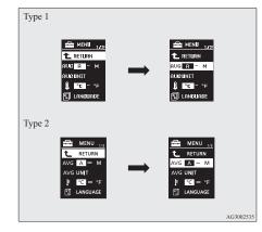
3. Press and hold the multi-information meter switch for about 2 seconds or more to switch in sequence from A or 1 (Auto reset mode)  $\rightarrow$  M, 2 or P (Manual reset mode)  $\rightarrow$  A or 1 (Auto reset mode).
