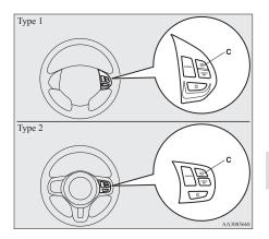
To increase your speed in small amounts, press the "ACC RES" switch for less than about 1 second and release it.
