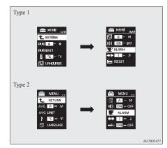
3. Press and hold the multi-information meter switch for about 2 seconds or more to display "ALARM" (rest time setting).
