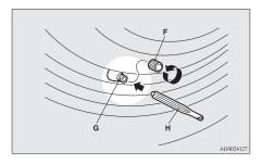
9. Remove the valve insert (I) by turning it anticlockwise using the valve remover (H). Put the removed valve insert in a clean place so it does not get dirty.
