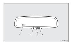
When the ignition switch is turned to the "ON" position, the green indicator (1) illuminates and the reflection factor of the mirror is automatically changed.
