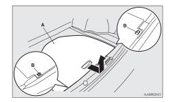
2. To remove the spare tyre, remove the installation clamp (C) by turning it anticlockwise.
