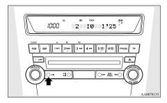
Push the CD button (2) if the discs are already in the autochanger. The autochanger will enter CD mode and start playback. The disc number, the track number and the playing-time will appear on the display. The discs in the unit will be played consecutively and continuously.
