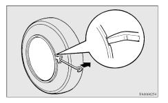
With the cover raised a little, pry it off completely using the jack bar. Insert the jack bar under the cover, and move it around the circumference, prying the cover away from the wheel little by little as you move the bar around.
