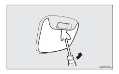
2. While holding down the tab (A), pull out the bulb.
