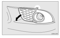
3. Remove the screws (B) and pull the entire lamp unit out.
