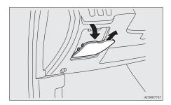
2. On vehicles with bottom cover, use the puller to loosen the 2 clips (A) and push down the bottom cover. The puller is in the fuse box in the engine compartment. Refer to "Fuse replacement" on page 8-26.
