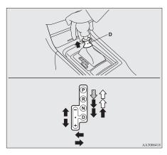
The pull-ring (D) must be pulled up while the brake pedal is depressed to move the gearshift lever.
