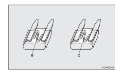
B- Fuse is OK C- Blown fuse
