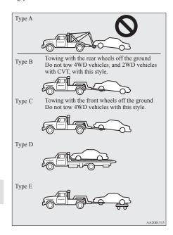
Towing the vehicle by a tow truck
