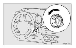
For vehicles with an A/T, CVT or Twin Clutch SST, when removing the key, first set the selector lever (A/T or CVT) or gearshift lever (Twin Clutch SST) to the "P" (PARK) position, and then turn the key to the "LOCK" position and remove it.
