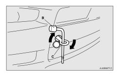
4. Secure the tow rope to the front towing hook.
