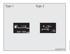
This displays the approximate driving range (how many more kilometres or miles you can drive). When the driving range falls below approximately 50 km (30 miles), "---" is displayed. Refuel as soon as possible.
