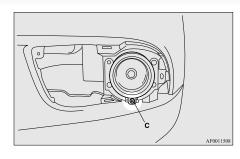
4. Push the connector (D) to disconnect and remove the fog lamp.
