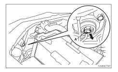
2. Remove the sealing cover (B).
