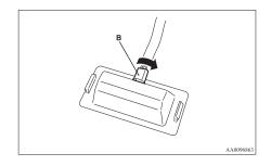
3. Remove the bulb by pulling out.
