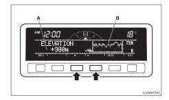
"+"- Adjustment of elevation
