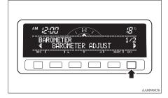
2. Press the "←" or "→" function button to select the "BAROMETER ADJUST" display. Then press the "SELECT" function button.
