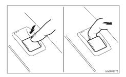
If the switch is fully pressed down/pulled up, the door window automatically opens/closes complete-
