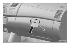
Type 2 The glove box can be locked and unlocked using the key.
