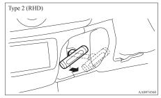
A- Parking brake lever stroke Type 1 8 to 9 notches Type 2 11 to 13 notches (Parking brake adjustment when pulled with the force of 200 N)
