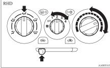
• For maximum heat, set the blower speed at the 3<sup>rd</sup> position.
