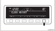
2. It is possible to adjust the clock using the function buttons.
