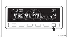
Press the "←" or "→" function button to select the setting you wish to adjust (daytime or nighttime). Then press the "SELECT" function button.
