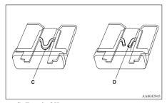
C- Fuse is OK D- Blown fuse
