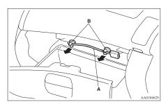
3. Connect the USB memory device (C) to the connector cable (A).
