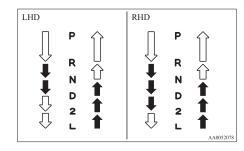
Lock button must be pushed to move the selector lever.
