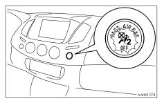
When the front passenger's airbag ON-OFF switch is turned OFF, the indication lamp will stay on to show that the front passenger's airbag is not operational.
