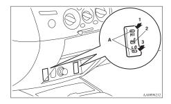
1 (HI)- Heater high (for quick heating).
