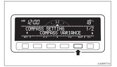
2. Press the function button for "←" or "→" to set the desired declination.
